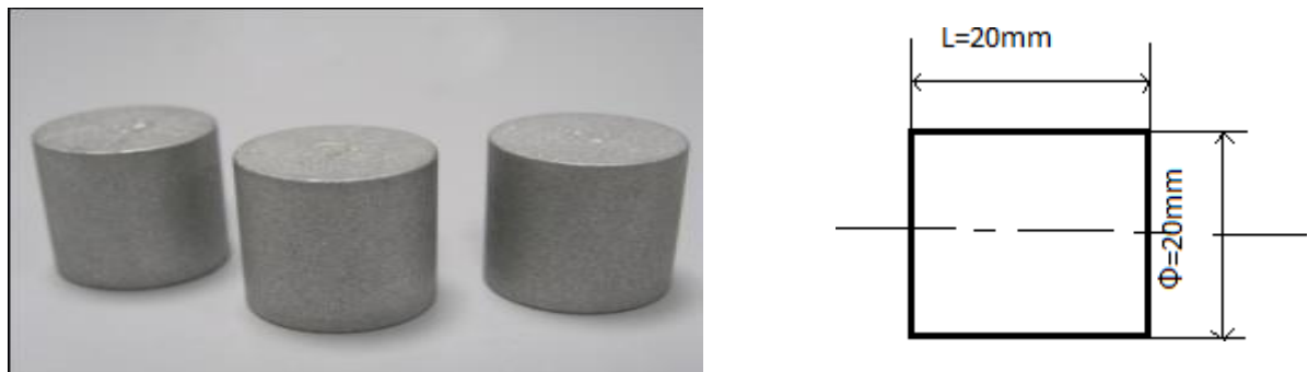
Figure 4 Roughness measured samples.
